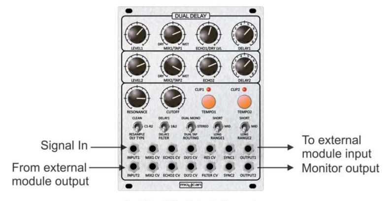
Set Dry/Wet1 to fully wet Level 2 controls feedback amount Set Dry/Wet 2 to fully Dry.
