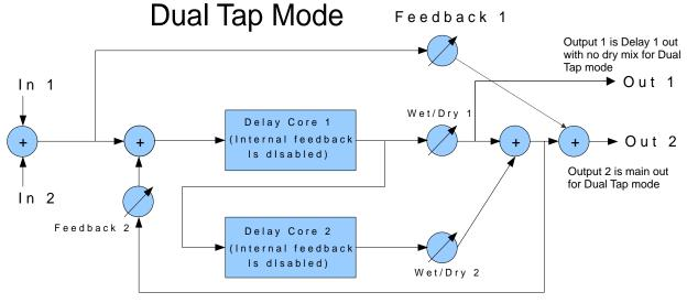
Note: In this mode the Wet/Dry controls are re-purposed as levels for each of the delay outputs. ECHO 1 becomes the dry signal level control and ECHO 2 sets the depth of feedback for the summed delays.
