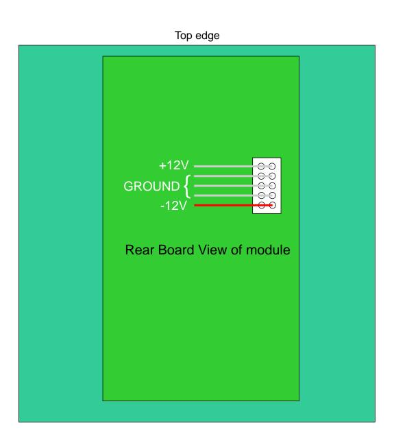
Place RED wire of ribbon cable so that it is connected to pins shown above
